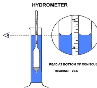
Make your best estimate when taking readings, as a hydrometer is a very finely graduated tool. I find the meniscus dip roughly equals 0.002 on the specific gravity scale.
